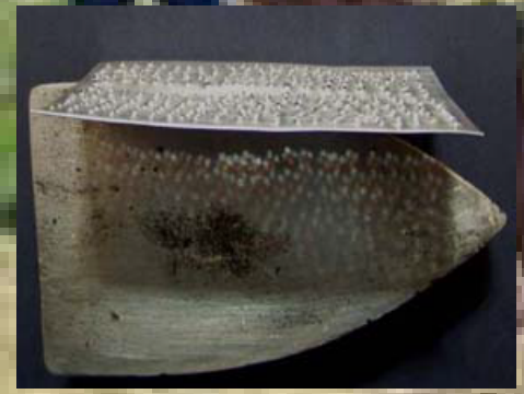
The rough interior working surface of the debarking tool.
